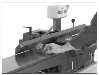
Figure 47. Adjusting fence 45° inward.
